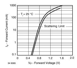
Figure 2. Forward Current vs. Forward Voltage
