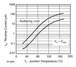
Figure 1. Reverse Current vs. Junction Temperature
