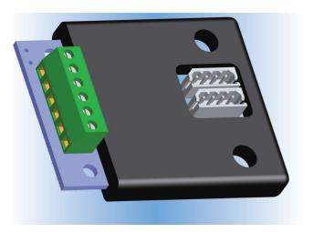
The EC Fan Controller is designed to operate without the use of an external power supply; using an ebm-papst patented design the controller draws its power from the 10V PSU integrated in the ebm-papst EC fan (10V, < 1mA).
