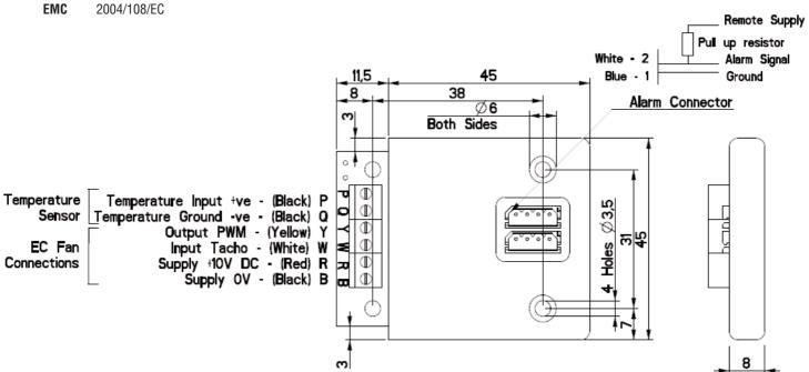
Note: for ebm-papst EC fans without an integrated 10 volt supply, please refer to the EC Fan Controller User Guide (980-OMI10740) for alternative wiring of the supply.
