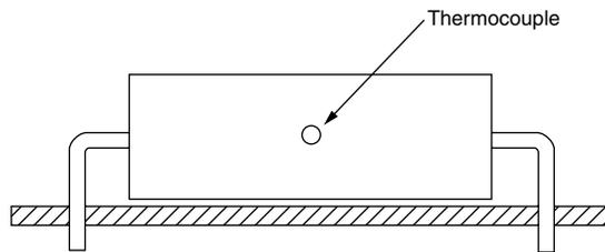
The temperature is measured in unloaded ( $T_{\text{amb}}$ ) and maximum loaded condition ( $T_{\text{C}}$ ).
