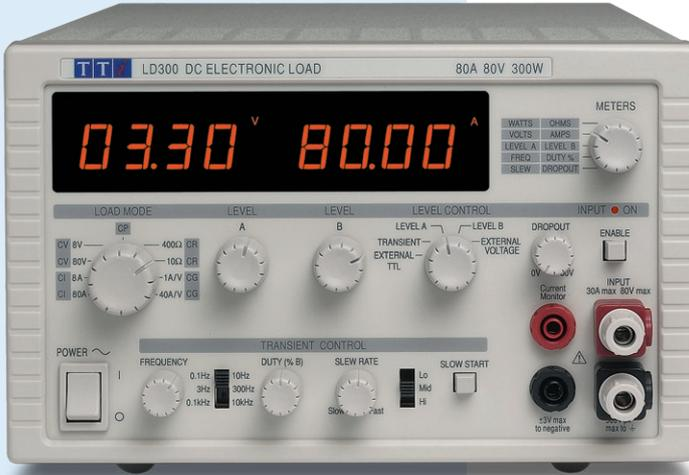
The LD300 is an inexpensive electronic load which is suitable for testing and characterising a wide variety of dc power sources.
