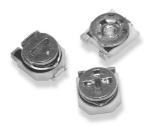
These cermet element surface mount trimmers feature a cross-slot adjustment head with unbroken perimeter for ease of vacuum pick up and auto adjustment.
