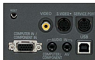
PLC-SW30 Terminal Input Panel
