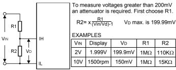
The input impedance becomes R1+R2. Choose accurate stable resistors. Typically, R1=1M $\Omega$ . 9M $\Omega$  is a practical upper limit.
