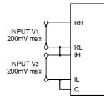
To determine the ratio between two voltages apply the inputs as shown. Displayed reading =  $\frac{V2}{V1}$  X 1000
