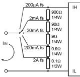
For multi-range, use, a 2 pole, 5 way rotary switch. 1 pole for range select and the other to connect the appropriate decimal point to XBP
