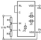
Using the formulae choose resistors to -O ensure the analogue inputs are no closer than 1.5V from either VDD or VSS (VDD-1.5V or VSS+1.5V)
