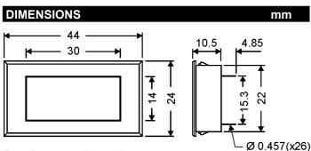
Panel cut out 40.5 x 22.5 Fastening clips accept panel thickness 0.9 to 3.2mm
