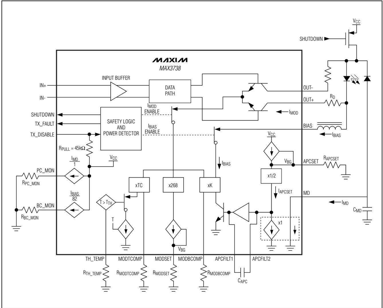
Figure 4. Functional Diagram
