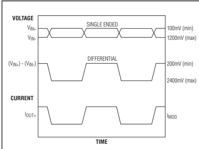
Figure 1. Required Input Signal and Output Polarity
