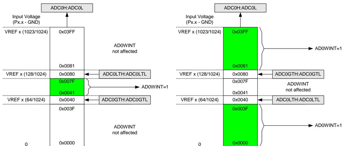
Figure 5.6. ADC Window Compare Example: Right-Justified Single-Ended Data
