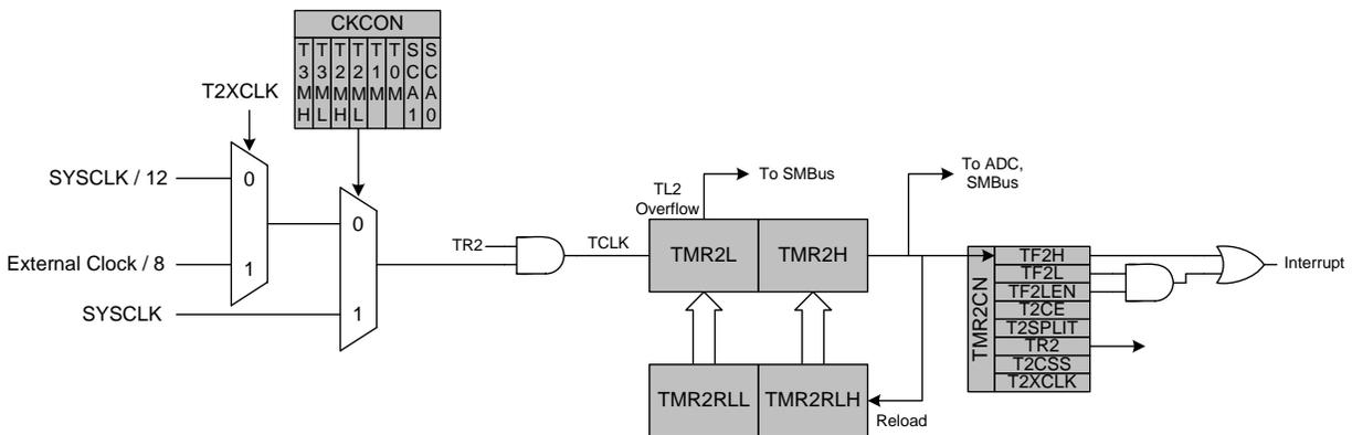
Figure 21.4. Timer 2 16-Bit Mode Block Diagram
