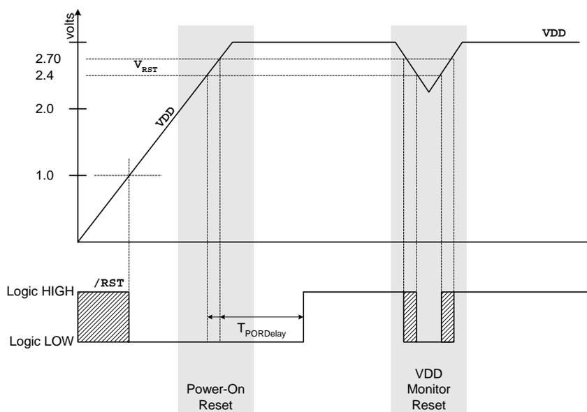
Figure 11.2. Power-On and  $V_{\text{DD}}$  Monitor Reset Timing
