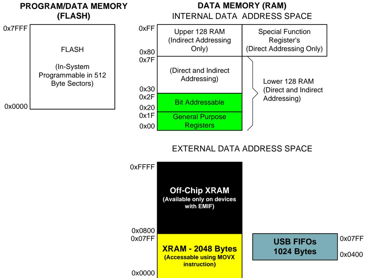
Figure 1.7. On-Chip Memory Map for 32 kB Devices (C8051F341/3/5/7/8/9)
