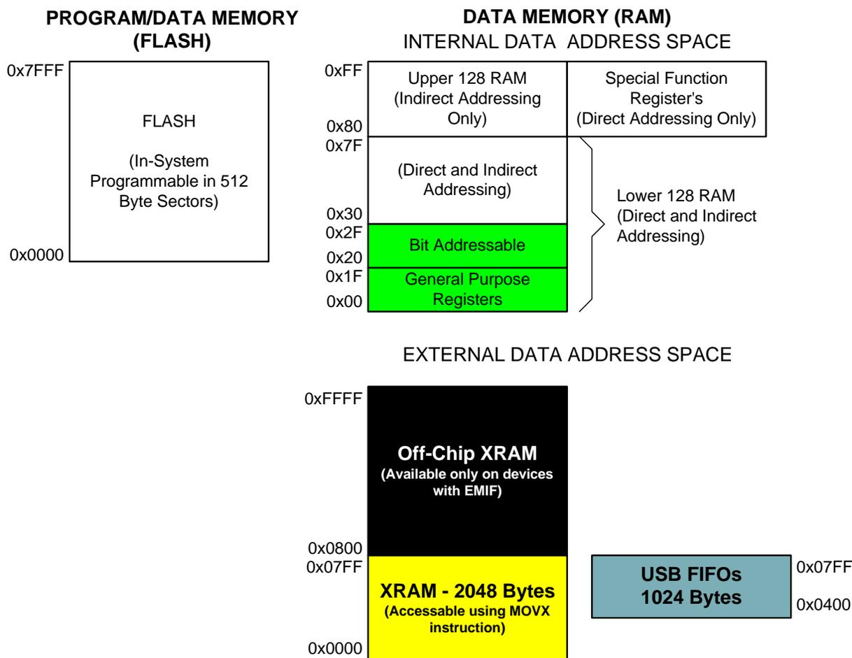
**Figure 9.3. On-Chip Memory Map for 32 kB Devices (C8051F341/3/5/7/8/9)**
