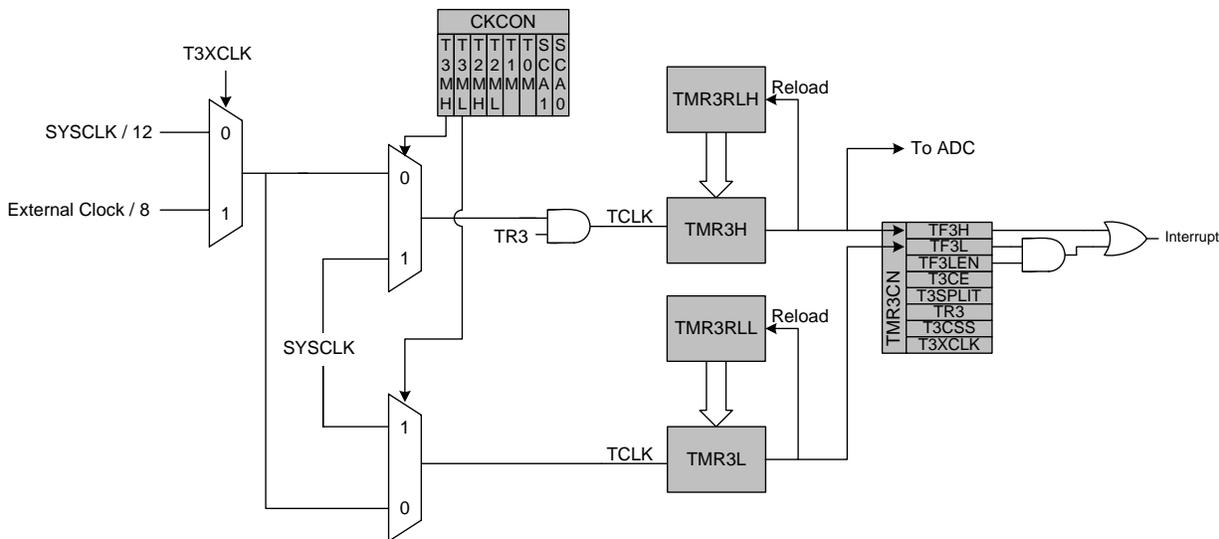
Figure 21.9. Timer 3 8-Bit Mode Block Diagram
