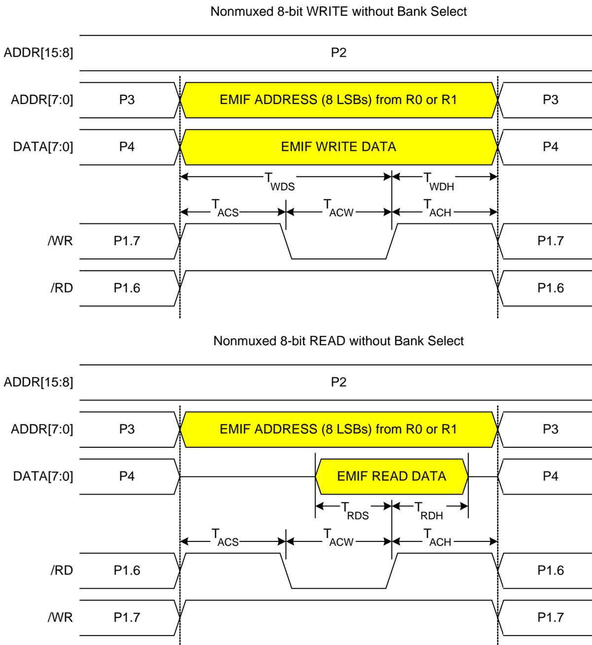
**Figure 13.6. Non-multiplexed 8-bit MOVX without Bank Select Timing**
