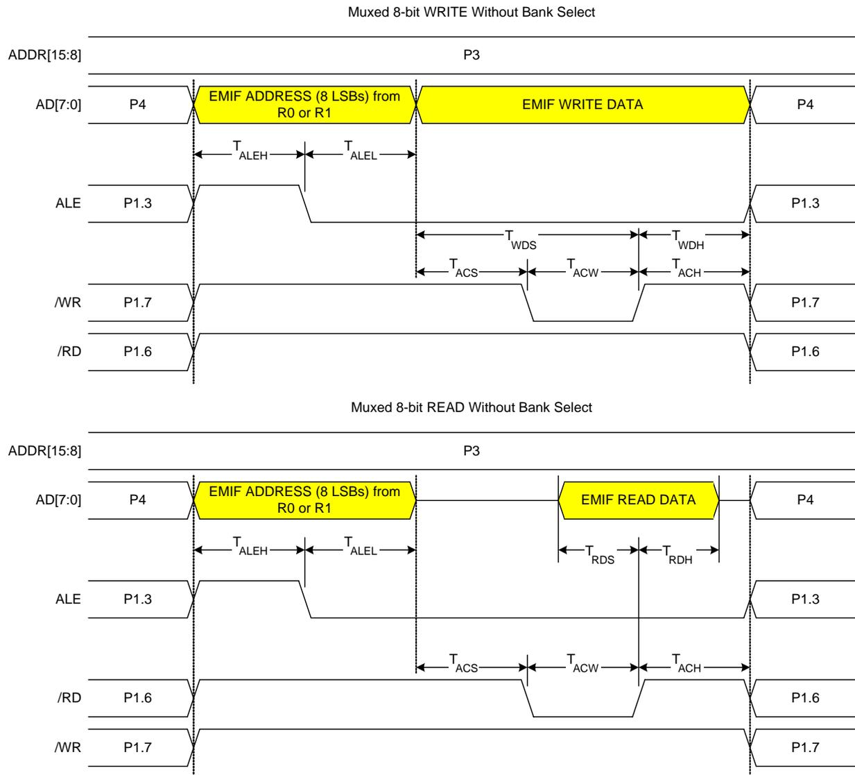
**Figure 13.9. Multiplexed 8-bit MOVX without Bank Select Timing**
