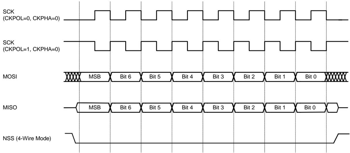
**Figure 20.6. Slave Mode Data/Clock Timing (CKPHA = 0)**
