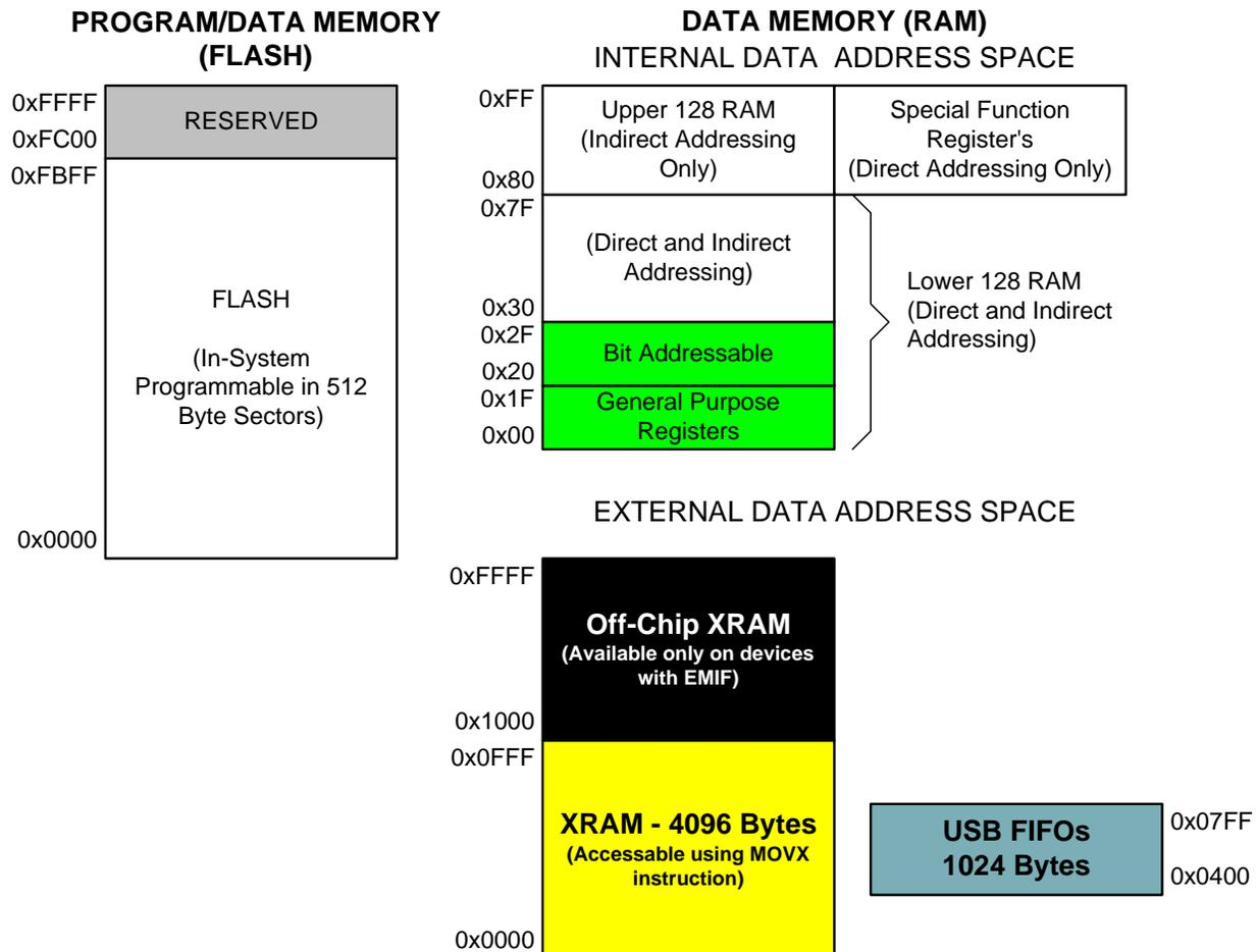
Figure 1.6. On-Chip Memory Map for 64kB Devices (C8051F340/2/4/6)
