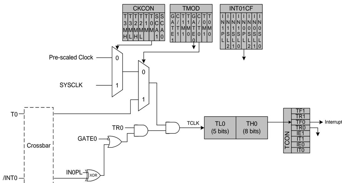
Figure 21.1. T0 Mode 0 Block Diagram
