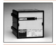
Manufactured to BS5685, IEC521 with a class accuracy of 1% to IEC1036, and supplied in a 96 x 96mm DIN case. The product has a 7 digit non resettable mechanical counter.
