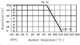
For temperatures in excess of 70°C the load shall be derated in accordance with the following figure.
