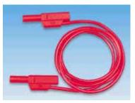
Flexible 1m length PVC connecting leads fitted with 4mm plugs. The slimline stackable plugs feature fixed shrouds and insulated tip centre pins for additional safety. Manufactured to **IEC1010-1**, **VDE0100/0110**, approved by **BG**. Working voltage 1000V, maximum current 32A.
