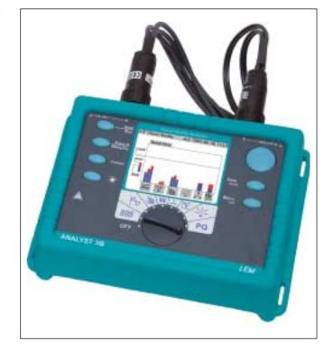
**ANALYST 3QC** is an ideal troubleshooting tool to identify and quantify power quality problems that effect the performance and efficiency of electrical plant and equipment.
