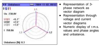
Simultaneous display of current and voltage vectors in colour with phase angle information for phase to phase voltage, phase to phase current and phase voltage and current.
