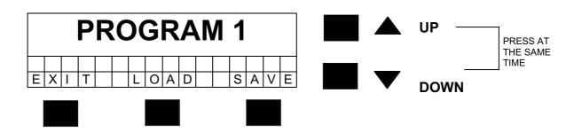
The program memories 1 - 10 can be selected using the **UP/DOWN** Control Keys (2)/(3).
