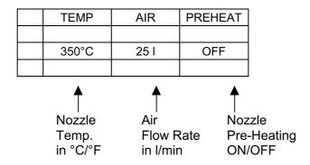
In the Manual operating mode the parameters for the nozzle temperature, air flow rate and switching on or off the pre-heating can be set.
