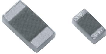
FC series chip resistors are designed with low internal reactance. They function as almost pure resistors on a very high range of frequencies. The specialized laser edge trimming allows for precision tolerances to 0.1 %.
