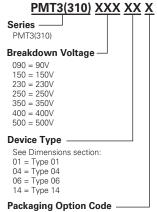
Blank = No Failsafe F = With Failsafe
