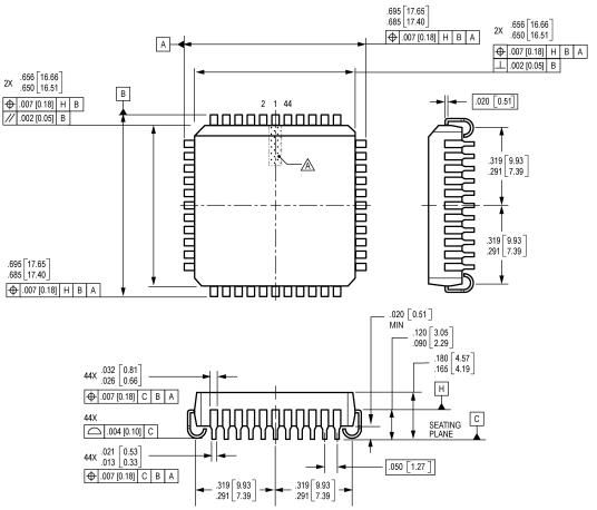
Preliminary dimensions, for reference only (reference JEDEC MS-018 AC) Dimensions in inches
