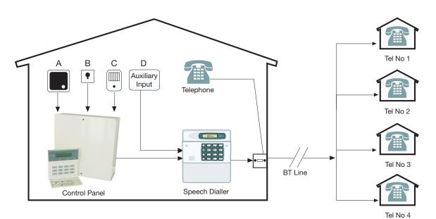
The SD1+ speech dialler accepts up to 4 inputs as shown in the diagram.
