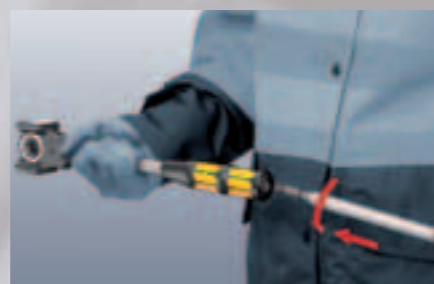
Here the extension can be used for better leverage
