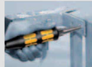
Tapered pin for aligning and centring
