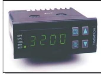
The TT32 programmable timer, packaged in a compact 75 x 33 x 69 mm housing, is an extremely versatile product offering nine operating modes applied to two timed output relay contacts. When only one of the timers is being used, the other output acts as an instantaneous set of changeover contacts. The single model provides timing from 0.1 seconds to 100 hours.
