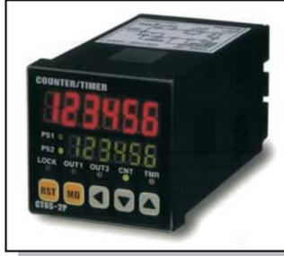
The CT range of counter timers has wide functionality at a competitive cost. Versions are available with 24-60Vdc and 100-264Vac power supplies, 4 or 6 digit dual LED displays and with 1 or 2 presets. The counter has 11 preset modes of operation including batch and cumulative. The timer has 9 modes including delay on, delay off, interval and cycle timer. The CT is housed in a 1/16 DIN 48 x 48mm case with an IP65 environmental rating.
