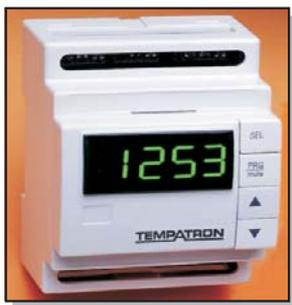
The TTDR timer has all of the features of the TT32 timer in a DIN rail mounting package. The TTDR covers time ranges from 0.1 seconds to 100 hours in a single model and has nine operating modes, two power supply options and two timed relay outputs. When only one timed output is being used the other output acts as an instantaneous set of changeover contacts. The TTDR matches the IRDR temperature controller on page 19.
