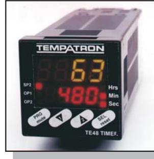
The TE48 is a panel mounting or plug-in programmable timer, packaged in a 1/16th DIN IP65 rated housing and is an extremely versatile product offering 11 operating modes applied to two timed output relay contacts. When only one of the timers is being used, the other output acts as an instantaneous set of changeover contacts. A single model provides timing from 0.1 seconds to 100 hours.
