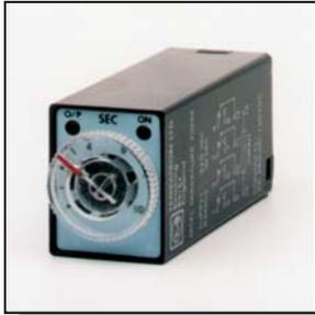
The MT4L series are miniature, 4 pole relay output, analogue timers operating in a 'Delay-on-Energise' mode only. They Offer a range of times and four standard voltages.
