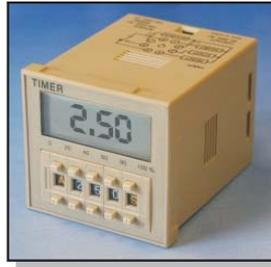
The LE3S timer has 10 operating modes and 10 time ranges, all selectable from the front panel. The LCD display shows the state of the output and a bar graph of the timing cycle as well as the 3 digit process time display. The single model is powered from 100 to 240Vac or 24 to 240Vdc. The LE3S is housed in a compact 1/16 DIN 48 x 48 mm case.
