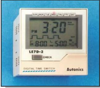
The LE7D is an electronic alternative to the mechanical time switch. It has two independent output relays that can each be programmed with 24 on-off, cyclic or pulsed steps for any combination of days within a weekly cycle. Housed in a 1/6 Din 72 x 72mm case, the LE7D has a clear LCD display and uses simple, intuitive programming techniques. All the programmed data is retained in memory even in the event of power failure.
