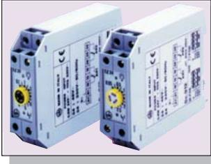
The TZ range of timers are designed for standard DIN rail mounting. With up to 2 DPCO relay outputs and operating voltages from 12Vac/dc up to 240Vac the TZ series is an economical solution to in-panel timing requirements.
