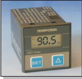
The UDT is a multi-function, multi-time range, digital timer which may be powered from 18 to 264Vac or dc. This single product is therefore suitable for almost any industrial application including those driven from 24Vdc batteries such as diesel generators, pumps, and back-up supplies. An internal Lithium battery ensures that user settings are retained in the event of power failure and, because of its low power consumption, the UDT can be programmed without a supply prior to installation.
