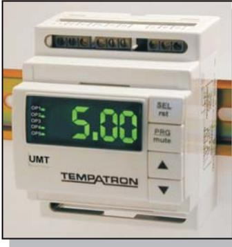
The UMT 500 timer is a programmable digital timer with 5 relay outputs, each of which has 5 selectable operating modes and an external start/reset function. Each output can either be programmed in timed or instantaneous mode making the UMT500 a particularly flexible unit for in-panel machine control applications that do not warrant the cost or complexity of an industrial plc.
