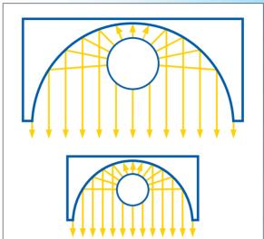
With the luminaire reflector reduced in proportion to the reduction in tube diameter, the shading effect remains the same. With the same luminaire efficiency, this gives designers enormous freedom to create new systems.
