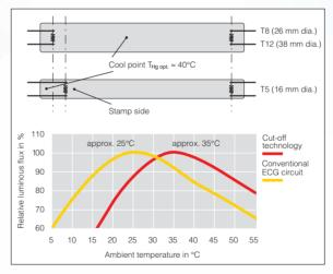
Luminous flux and temperature behaviour of T8 (26 mm dia.) and T5 (16 mm dia.) with cut-off technology Optimum luminous flux at 35°C in the case of T5 (16 mm dia.) lamps can only be achieved with cut-off technology.
