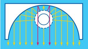
The diagram compares the shadowing effects caused by T8 and T5 lamps in a T8 reflector. The new FH® lamp with its diameter of only 16 mm represents a much smaller obstruction to the light rays than the 26 mm lamp, so less light remains trapped in the luminaire.
