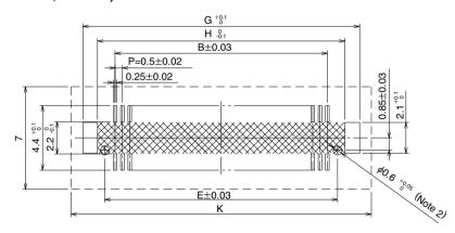
Note1: If the pattern is included in the shaded area, and is not treated with resist, it could touch the connector contact.
