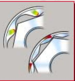
The Metrinch Wall Drive Profile was designed to provide a greater area of force application, compared with that applied by conventional tools. This profile, because of the buttress effect of its load bearing lugs, does not transmit the extreme peaks found when a tool with a wedge shaped profile is used. In distributing the torque load to the fastener through the flats, the Metrinch tool does not only achieve greater force, but also lowers the
