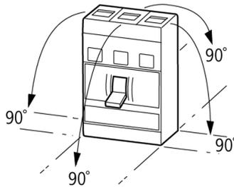
With plug-in adapter NZM2, N(S)2: vertical, 90° right/left
