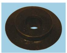
$\bf 155\text{-}4377$  - fits models 155-5786 and 162-3677. Suitable for cutting copper, brass, aluminium and light gauge steel pipes.
