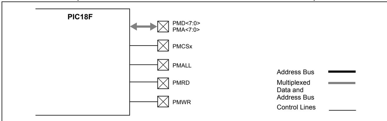
**FIGURE 11-11: FULLY MULTIPLEXED ADDRESSING MODE
