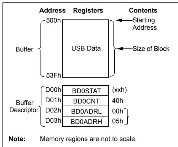
Unlike other control registers, the bit configuration for the BDnSTAT register is context-sensitive. There are two distinct configurations, depending on whether the microcontroller or the USB module is modifying the BD and buffer at a particular time. Only three bit definitions are shared between the two.
