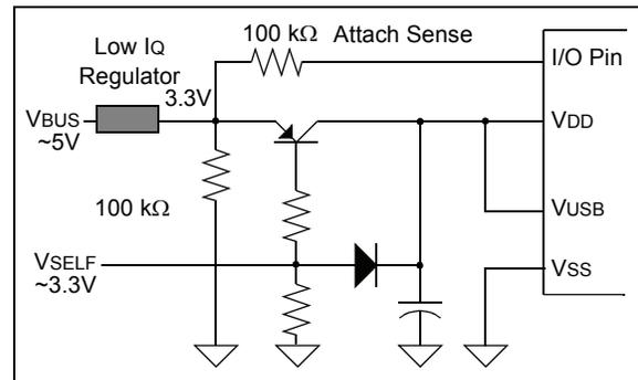
**Note:** Users should keep in mind the limits for devices drawing power from the USB. According to USB Specification 2.0, this cannot exceed 100 mA per low-power device or 500 mA per high-power device.
