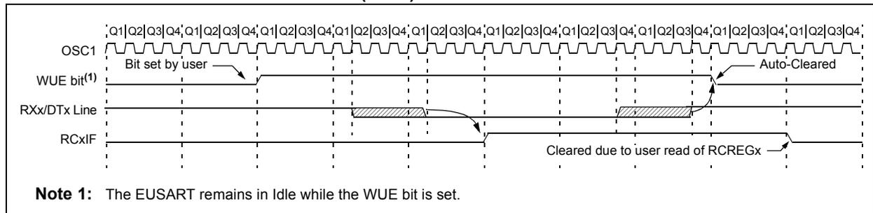
**FIGURE 21-9: AUTO-WAKE-UP BIT (WUE) TIMINGS DURING SLEEP**
