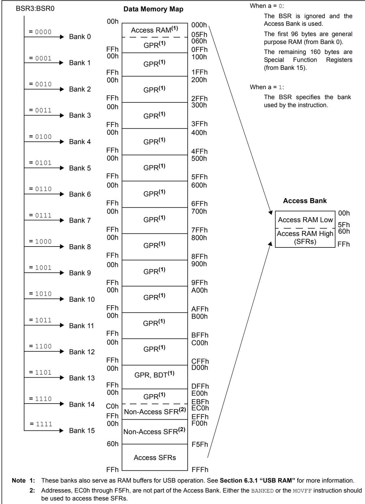
**FIGURE 6-7: USE OF THE BANK SELECT REGISTER (DIRECT ADDRESSING)**
