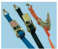
25mm ratchet load restraints (British made polyester webbing) are ideal for the lighter loads, for securing small pallets and the like. These assemblies come with claw hooks.
