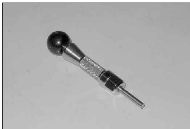
Extraction tool for contact # 12: 51 06 021 0924 Extraction tool tip: 51 06 021 3424
