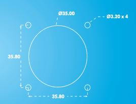
When mounted this way the panel acts as the bezel and no separate bezel is needed. M3 machine screws are recommended.
