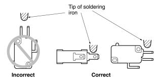
When soldering automatically, adjust the amount of solder so that flux does not float onto the top of PCB. If flux enters the switch, it can cause contact failure.
