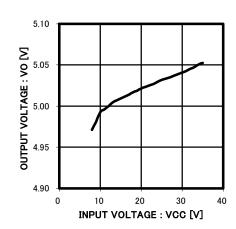
Fig.23 OUTPUT VOLTAGE-INPUT VOLTAGE (Vo=5V,Ro=5ohm)
