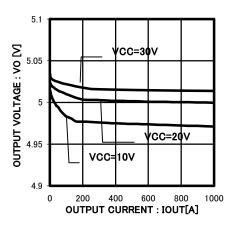
Fig.22 OUTPUT VOLTAGE-LOAD CURRENT
