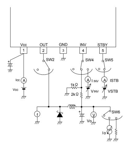
Fig.32 Input Output Measurement Circuit
