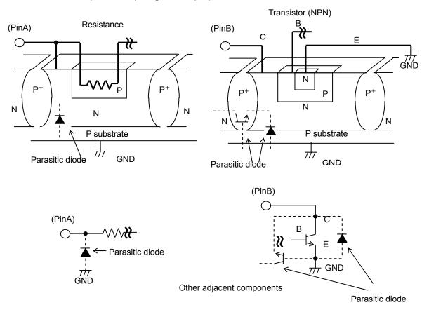
Fig.34 Simplified structure of a Bipolar IC
