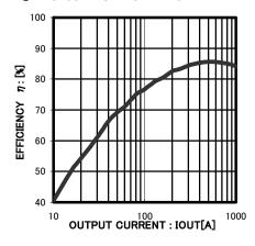
Fig.19 EFFICIENCY-LOAD CURRENT
