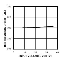
Fig.26 fosc-INPUT VOLTAGE
