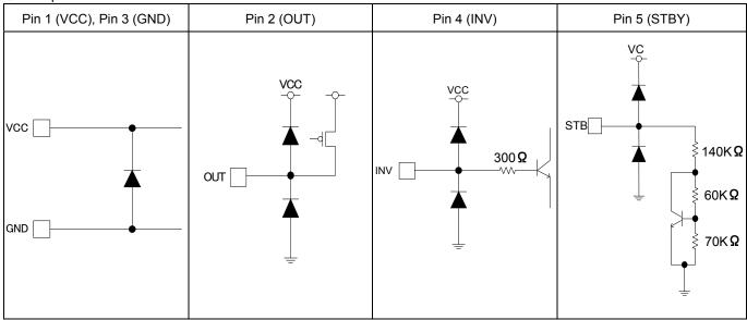
Fig.33Input Output Equivalent Circuit
