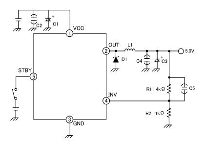
Fig.31 Recommended Circuit Output Voltage 5V: Application cicuit example
