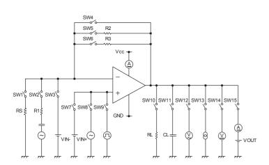
Fig.3 Measurement Circuit 2 (each Op-Amp)
