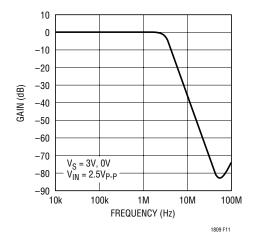
Figure 11. Filter Frequency Response
