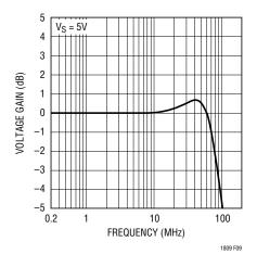
Figure 9. Video Line Driver Frequency Response
