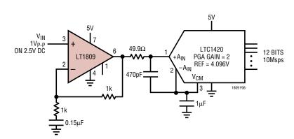
Figure 6. Single Supply A/D Driver
