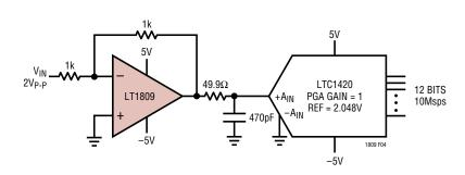
Figure 4. Inverting A/D Driver
