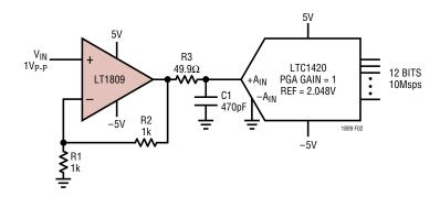
Figure 2. Noninverting A/D Driver
