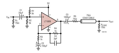
Figure 8. 5V Single Supply Video Line Driver
