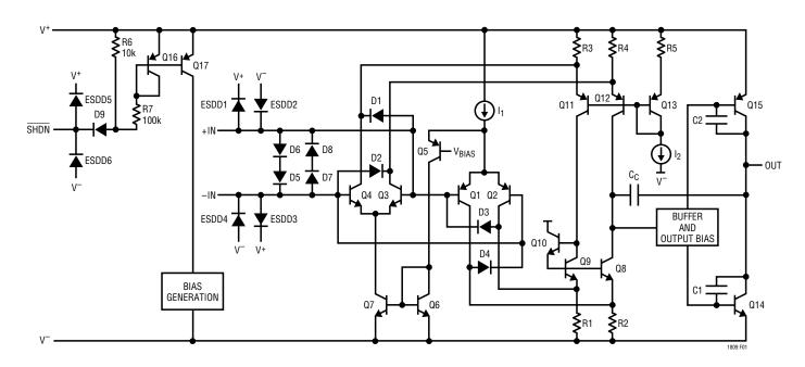
Figure 1. LT1809 Simplified Schematic Diagram
