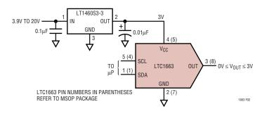
Figure 2. LT1460 As Power Supply for the LTC1663
