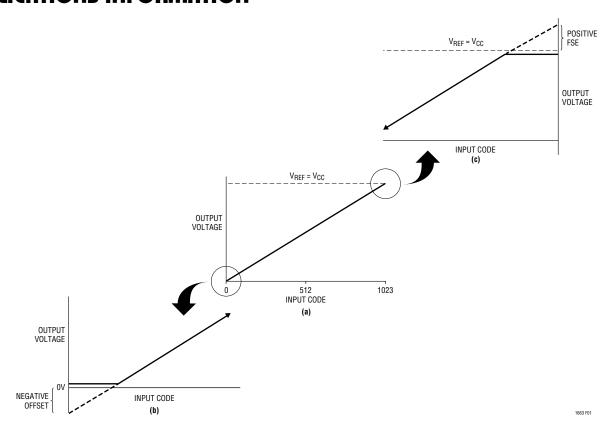
Figure 1. Effects of Rail-to-Rail Operation On a DAC Transfer Curve. (a) Overall Transfer Function (b) Effect of Negative Offset for Codes Near Zero Scale (c) Effect of Positive Full-Scale Error for Input Codes Near Full Scale When  $V_{REF} = V_{CC}$
