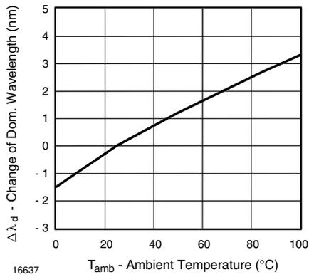
Figure 8. Change of Dominant Wavelength vs. Ambient Temperature
