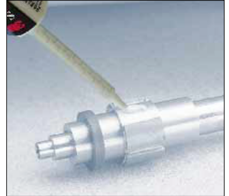
Bonding a magnet to a steel rotor 3M Scotch-Weld DP 460
