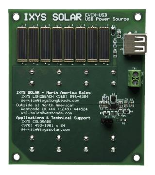
Eight series-connected SolarBITs convert sunlight to current and charge four AA cells connected in series/parallel for 3V. The converter IC boosts the battery voltage to +5V, available via a USB Series A receptacle and a screw terminal block. The AA cells will charge any time the Solar Bits are exposed to daylight. Move the push-on jumper from OFF to ON to operate the converter and generate +5V.
