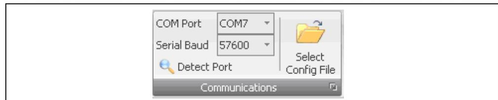
**COM Port** – Select the emulated serial communications port used by the hardware.
