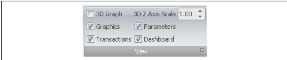
**3D Graph** – Check the box for the Graphics window to display a three dimensional map of the capacitance measurement values. Uncheck the box for Graphics window to display a two dimensional map of the capacitance measurement values.
