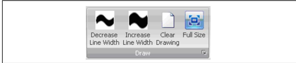
**Decrease Line Width** – Decreases the brush or line width used when drawing in the drawing window.
