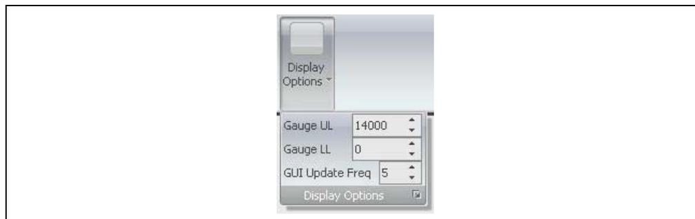
**Gauge UL** – Set the upper limit on the scaling in the Graphics window.
