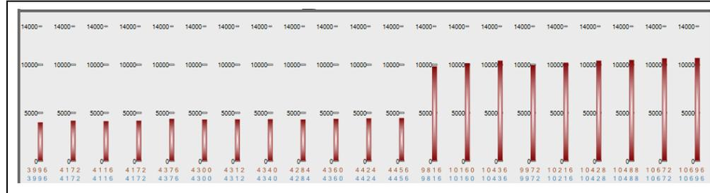
Each red bar on the graph represents the measured capacitance for a unique electrode on the sensor.
