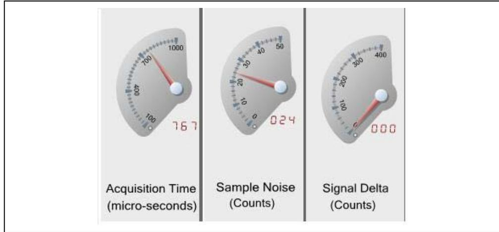
**Acquisition Time Gauge** – The Acquisition Time gauge displays how long the hardware is taking to measure the capacitance of a single electrode on the sensor. A shorter time is better because it means the hardware is able to measure the sensor in less time, yielding better touch responsiveness.
