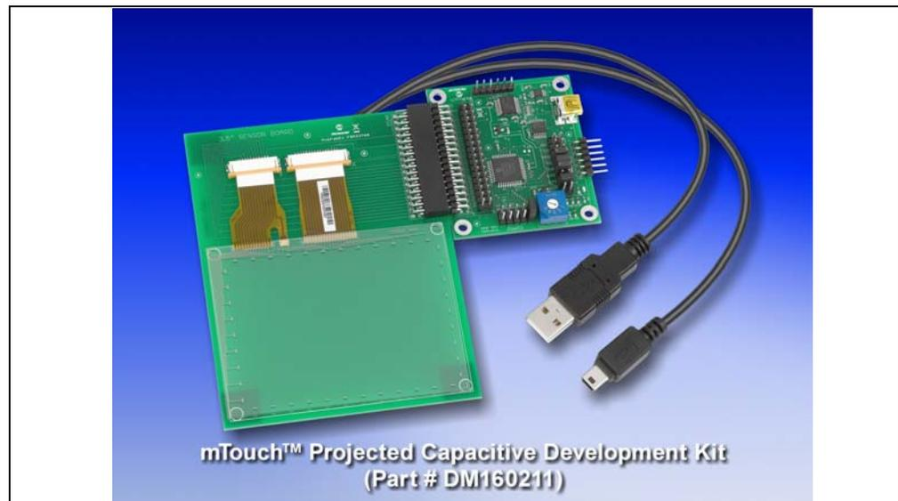
**Note:** This Evaluation Kit is intended as a functional evaluation of Microchip's mTouch Capacitive Sensing Solutions. It has not been designed for use in noisy or production-level testing environments.
