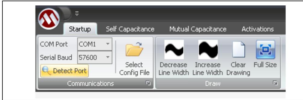
Touch and draw on the sensor to confirm if basic operation has been established. You should see your drawing motion reflected in the Drawing window of the Startup tab.
