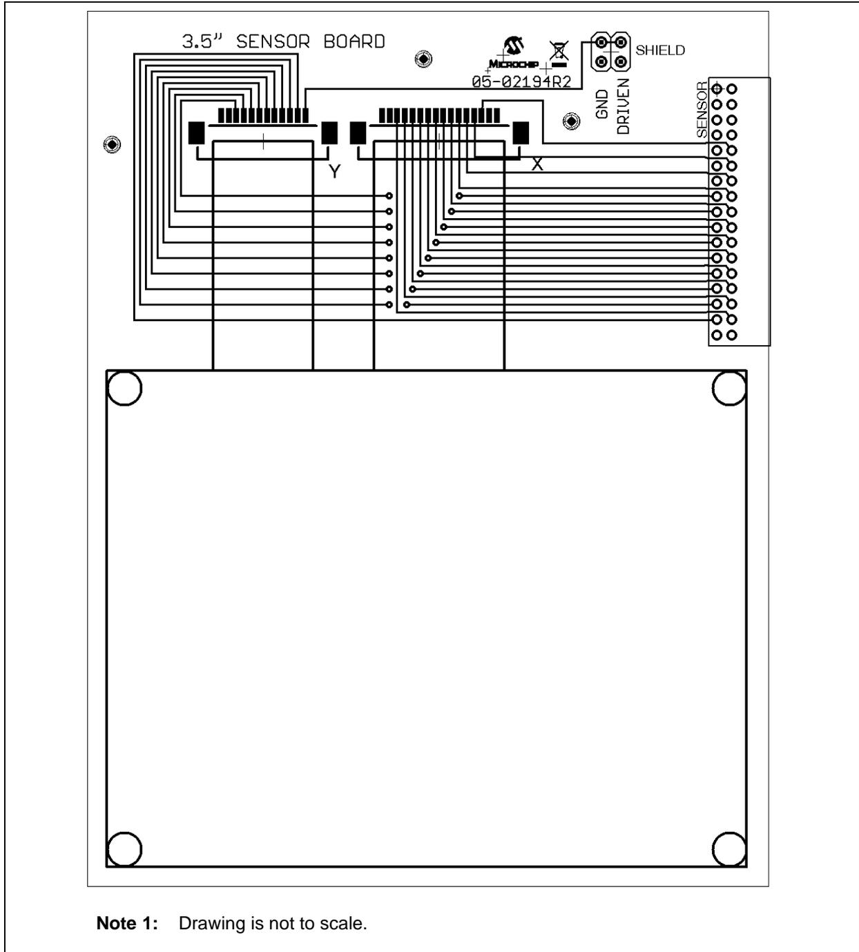
FIGURE A-3: PROJECTED CAPACITIVE BOARD SCHEMATIC
