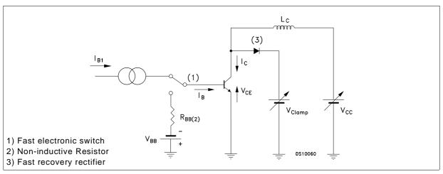
Figure 2: Resistive Load Switching Test Circuit.
