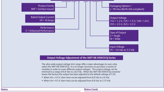
1 When Vin  $\ge$  4.5 V, then Vout can be adjusted from 0.8 Vdc to 3.6 Vdc. When Vin < 4.5 V, then Vout can be adjusted from 0.8 Vdc to 2.75 Vdc.
