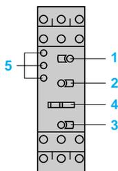
1 Potentiometer for fine adjustment of the time delay, graduated in % of range max. setting 2.
