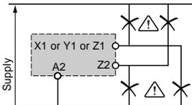
No galvanic insulation between supply terminals A1, A2, B1, B2 and control inputs X1, Y1, Z1, Z2.
