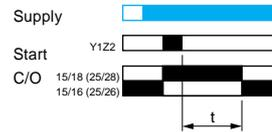
**Pulse on energisation relay with start on opening of the external control contact**
