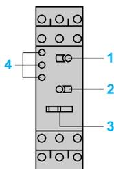
1 Potentiometer for fine adjustment of the time delay, graduated in % of range max. setting 2.
