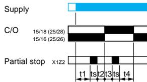
**Conversion of second changeover contact to instantaneous mode by means of switch R2**
