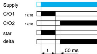
**External control for start of time delay (example on On-delay function) (1)**
