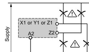
⚠ No galvanic insulation between supply terminals A1, A2, B1, B2 and control inputs X1, Y1, Z1, Z2.
