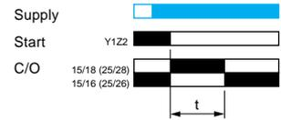
**Relay for star-delta starters with: double On-delay timing**
