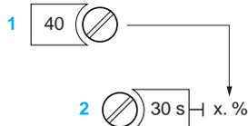
1 Potentiometer for fine adjustment of the time delay, graduated in % of range max. setting 2.
