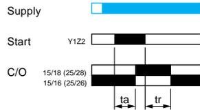
**Remote control for partial stop of time delay**
