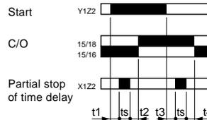
**Conversion of second changeover contact to instantaneous mode by means of switch R2**
