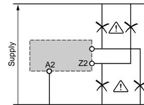
⚠ No galvanic insulation between supply terminals A1, A2, B1, B2 and control inputs X1, Y1, Z1, Z2.
