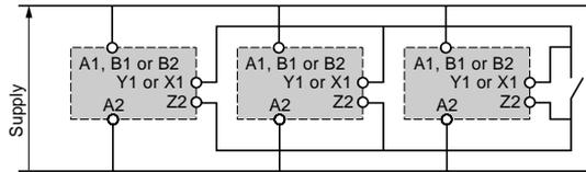
Connection of Telemecanique 3-wire NPN or PNP sensor
