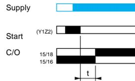
**External control for partial stop of time delay (example on pulse on energisation relay) (1)**
