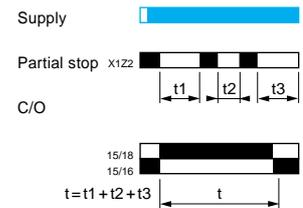
**Conversion of second changeover contact to instantaneous mode by means of switch R2**
