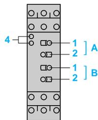
1 Potentiometer for fine adjustment of the time delay in % of range max. setting 2.
