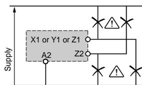
⚠ No galvanic insulation between supply terminals A1, A2, B1, B2 and control inputs X1, Y1, Z1, Z2.
