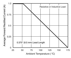
Figure 1. Forward Current Derating Curve
