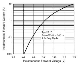
Figure 3. Typical Instantaneous Forward Characteristics
