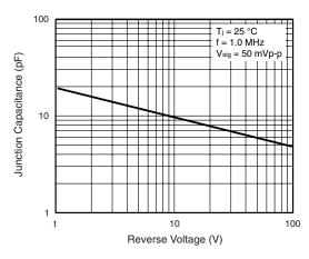
Figure 5. Typical Junction Capacitance
