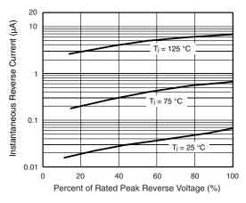
Figure 4. Typical Reverse Characteristics
