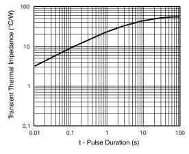
Figure 6. Typical Transient Thermal Impedance
