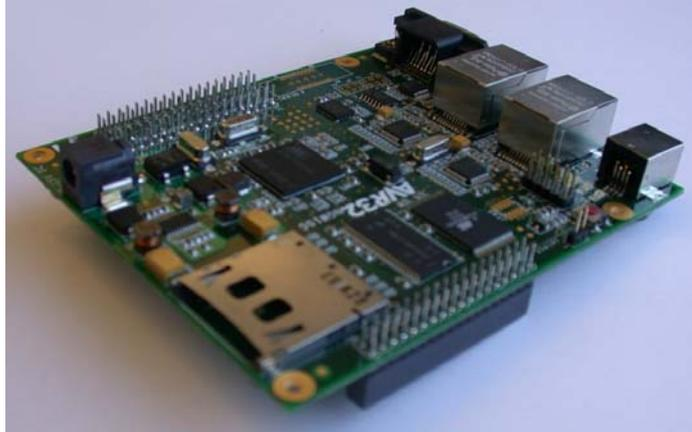
After inserting the stack through headers into NGW100 they must be soldered to the PCB. This is done by applying heat with the solder iron to the via and header pin and applying solder, see Figure 3-2. The solder should sink into the via to make a firm connection between the via and the header pin, see Figure 3-3 for an example solder.
