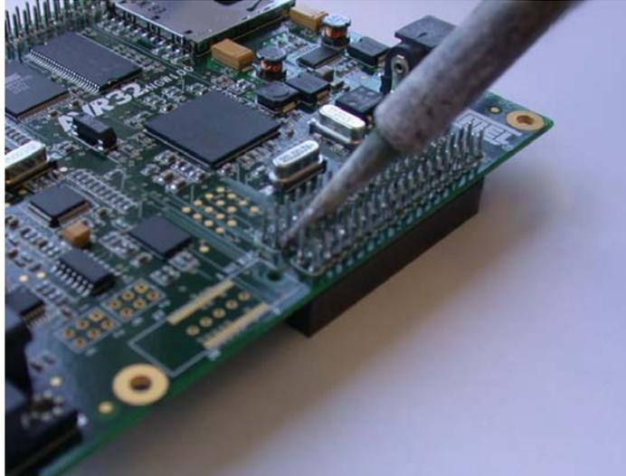
**Figure 3-3.** Example solder of a header pin to via on NGW100 PCB
