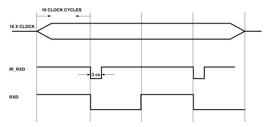
A high to low transition of the IR\_RXD line from the HSDL-1000 signifies a 3/16th pulse. This pulse is stretched to accommodate 1 bit time (16 clock cycles). Every pulse that is received is translated into a "0" or space on the RXD line equal to 1 bit time.
