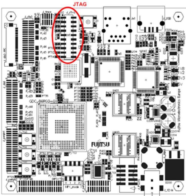
A Segger J-Link Arm Lite adapter is included. It is connected as shown in the picture below.
