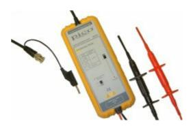
The TA041 is an active differential oscilloscope probe. The probe permits the measurement of signals which are not referenced to earth using a conventional earthed oscilloscope. This enables mains voltages to be tested. It is possible to measure and observe the waveforms of three phase supplies or the gate/control signals of semiconductor circuits. It is ideal for investigation of motor speed controls, uninterruptible power supplies, switch mode power supplies and process controllers.
