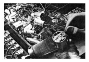
ALU-SOL 45D being used to join a tinned Copper Foil Tab to the aluminium can of a suppression filter at the Great Yarmouth Factory of ITT Components Group Europe. The speed and reliability achieved by using a gas torch and ALU-SOL is essential for this highly competitive market.
