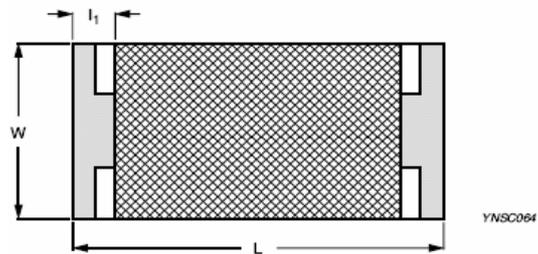
Fig.2 Chip resistor outlines
