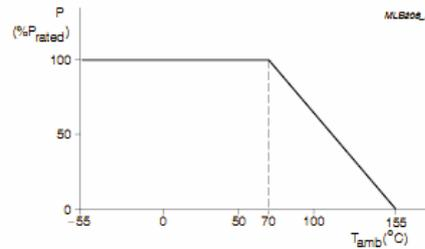
Fig. 3 Maximum dissipation (P) in percentage of rated power as a function of the operating ambient temperature (T<sub>amb</sub>)
