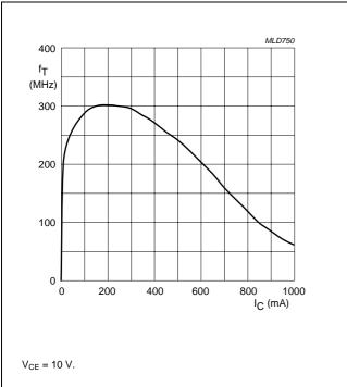
Fig.6 Transition frequency as a function of collector current.
